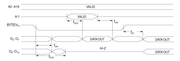
Notes: 1. Timing measurement references are 0.8V and 2.0V. Input AC drive levels are 0.45V and 2.4V, unless otherwise specified.
