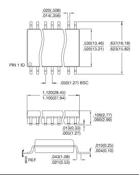
**48T**, 48-lead, 12 x 20 mm, Plastic Thin Small Outline Package (TSOP) Dimensions in Millimeters and (Inches)\* JEDEC OUTLINE MO-142 BD
