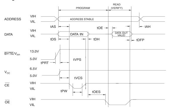
Notes: 1. The Input Timing reference is 0.8V for  $V_{\rm IL}$  and 2.0V for  $V_{\rm IH}$ .
